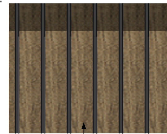
1.5 X 3/4" @ 1/4" DETAIL A Scale 1:8
