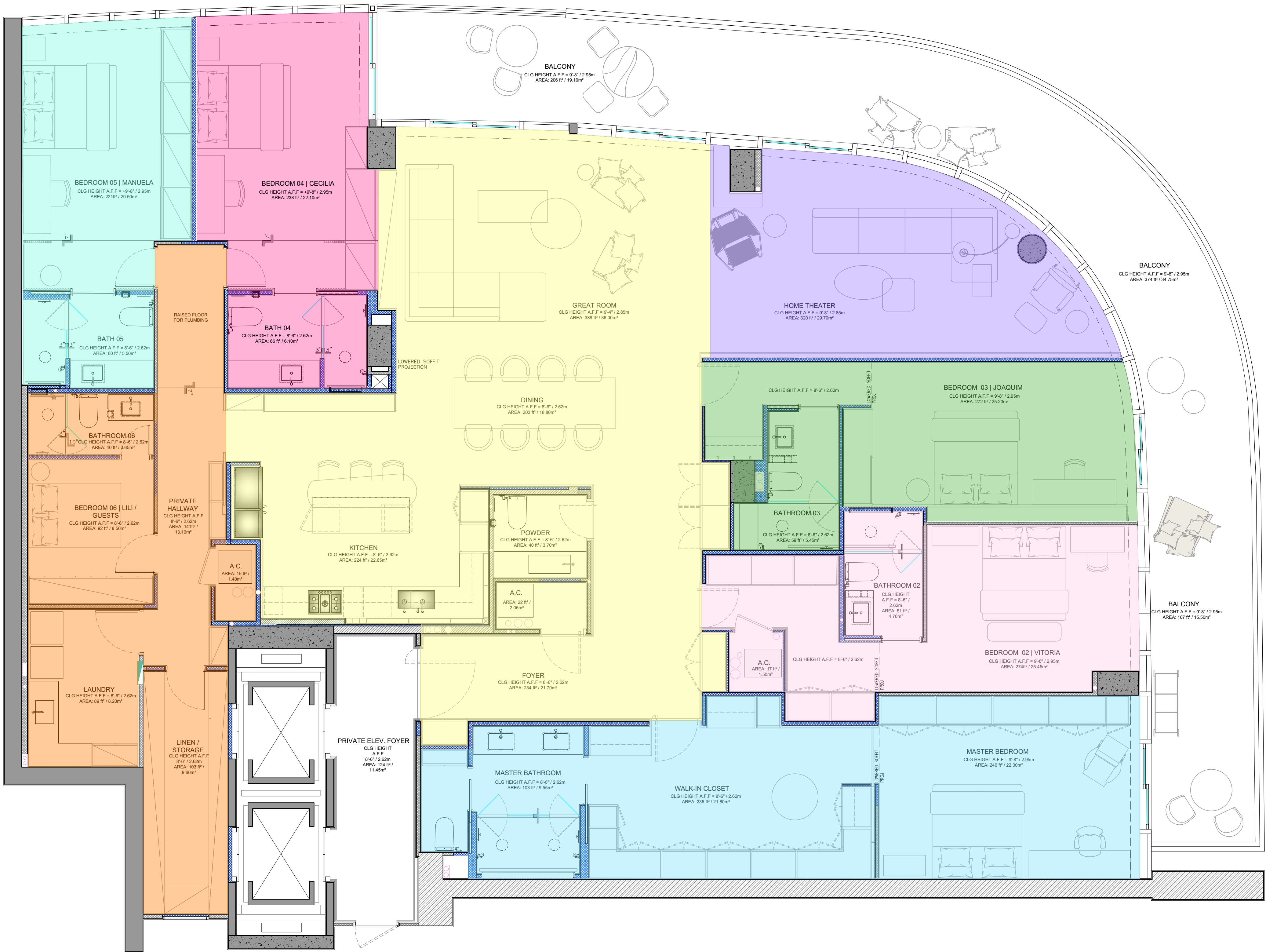
AIR CONDITIONING ZONES - PLAN scale 1:50
